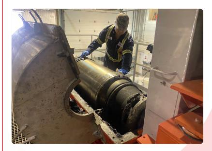
The new centrifuge at the Chatham, Ontario hazardous waste facility is designed to separate solid and liquid hazardous waste materials so they can be recycled or collected for proper disposal. It is the first technology of its kind to be used for hazardous waste management in Canada, and in its first year is already seeing great demand from area oil refineries and other customers.
